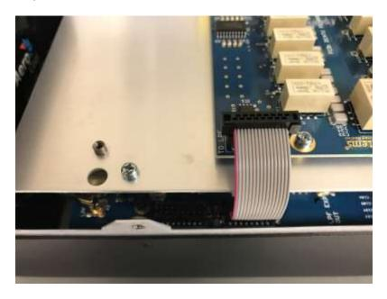
**Step 10:** Next install the RF shield plate with ATU board down on the standoffs and align with screw holes.
