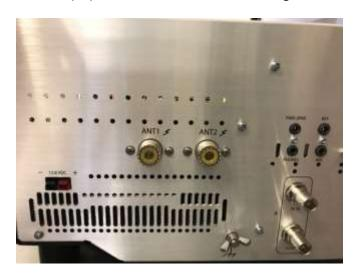
**Step 12:** The right angle coax connectors need to be connected to the ATU as shown below. Note: keep the short coax away from L1 as much as possible as shown in the picture.
