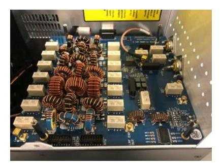
**Step 6:** Remove ATU from the bag and insert the two cables provided as shown. Both cables should be inserted from the top with the straight connector going through the grommet and the right-angle connector on top. The longer of the two cables goes through the grommet nearest the inductors with the most coils.
